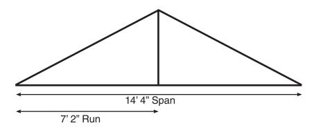
Note: Run is half the Span.
