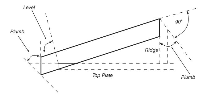
**Plumb:** Vertical Cut. The angle of cut from the edge of the board that allows the rafter to mate on the vertical side of the ridge rafter.
