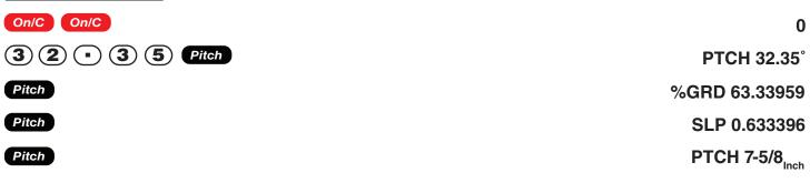
Note: To convert Pitch in Inches: Simply enter the Pitch in Inches first (e.g. () (Inch Pitch ) then continuously press the Pitch key to calculate the pitch conversions, as above.
