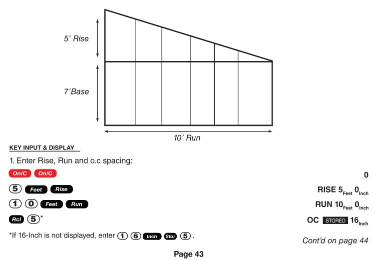
2. Enter base, then find stud lengths and angle of incline:
